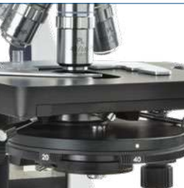
Zernike phase contrast condenser with filter holder
